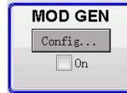
The internal modulation source is configured through this panel. An internal pulse generator can be used as a pulse modulation source.
