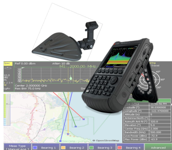
TDOA PC software KSMS calculates the intersection of the hyperbolas and determines the geo-location of the RF signal source
