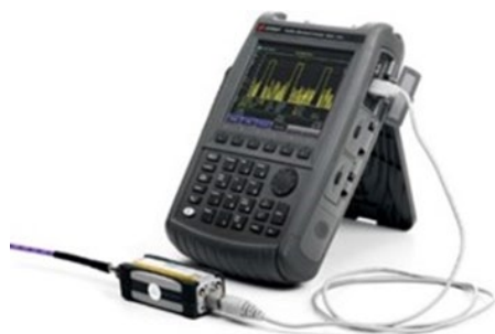
Simplify power measurements with USB power sensors
