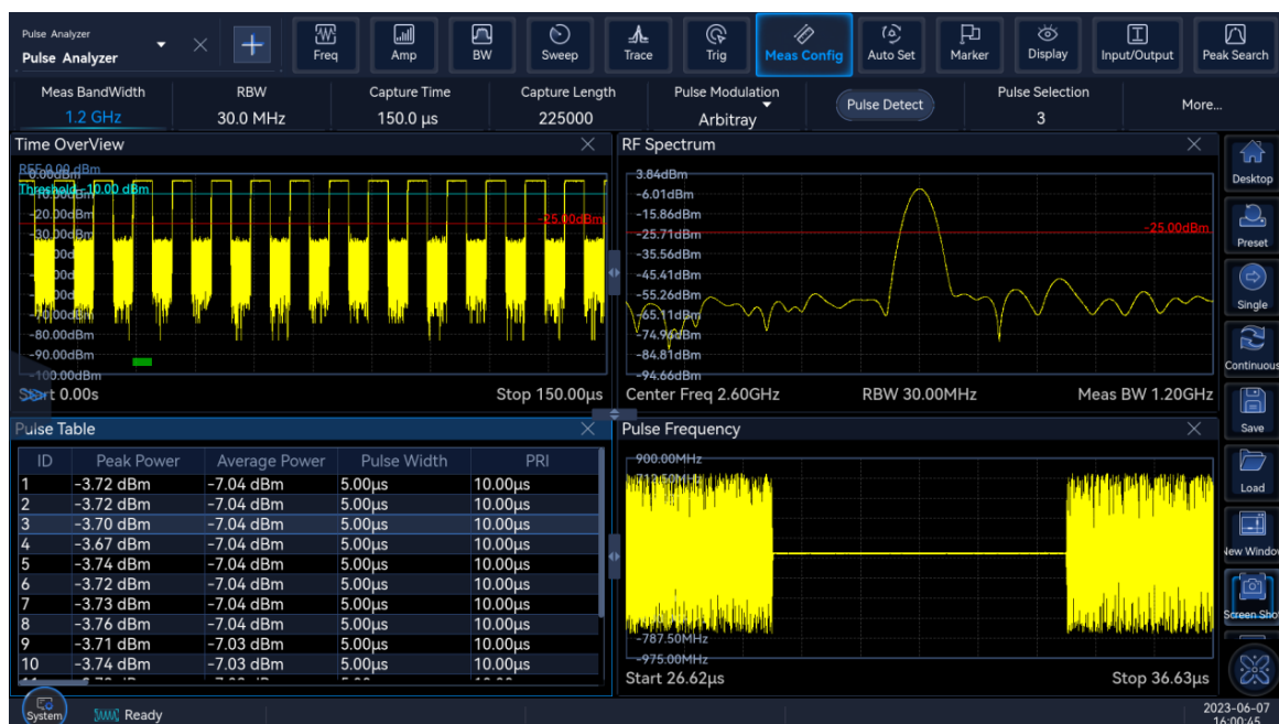
1.2GHz Analysis Bandwidth Measurement
