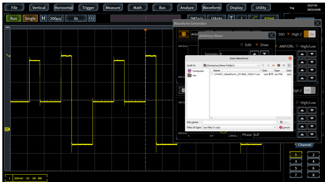
Stored waveforms are copied from the waveform generator.
