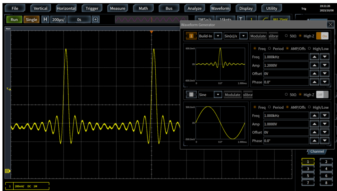
Built-in waveform output: SinC, exponential up-and-down, Gaussian, Lorentz curve, semi-positive curve
