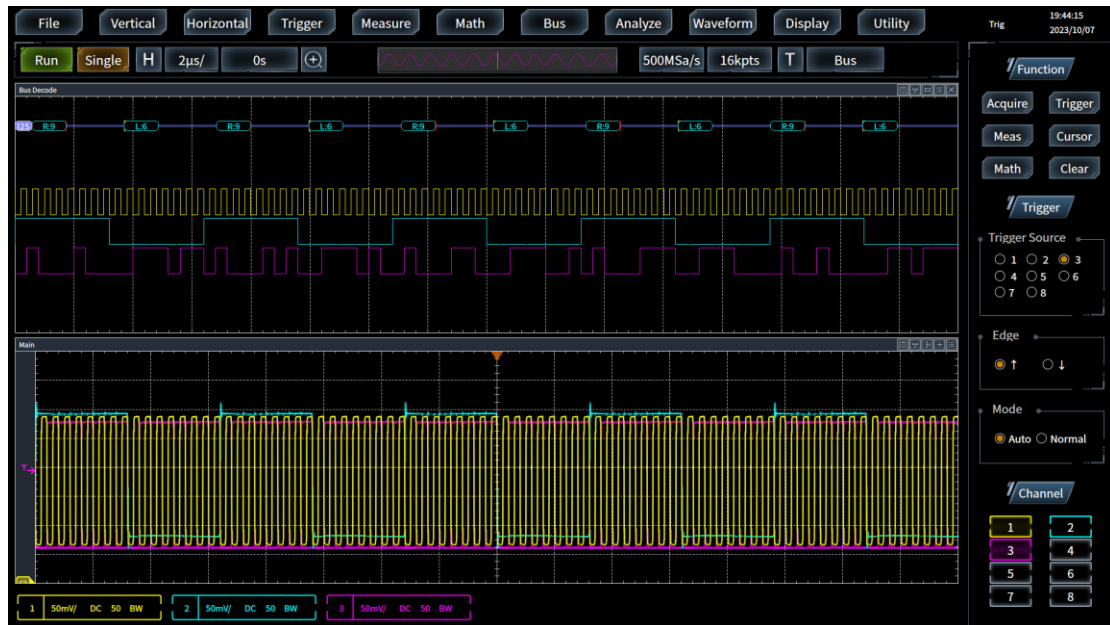
I2S, LJ, RJ, TDM audio buses
