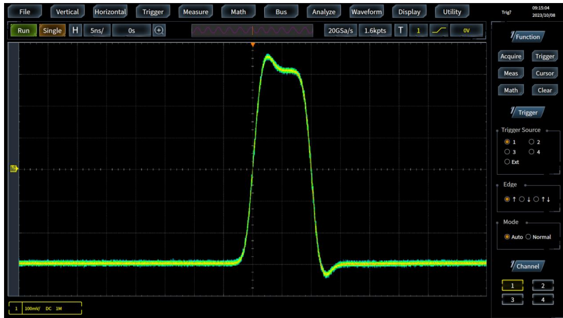
20GSa/s sampling rate helps to accurately reconstruct signal waveform
