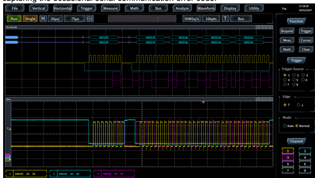
I2C, SPI embedded buses
