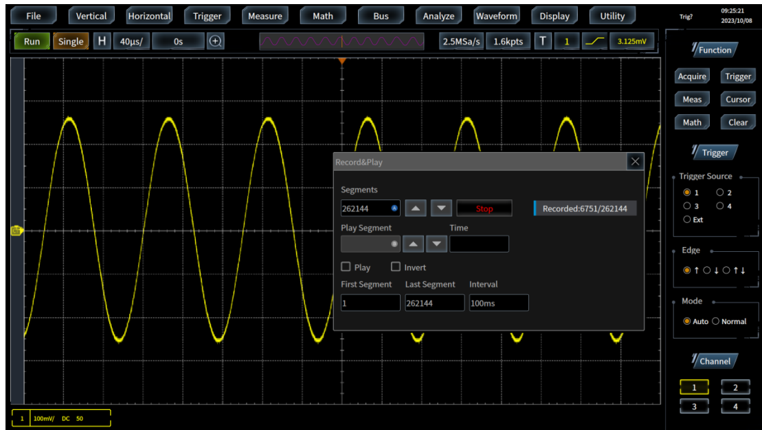
Segmented memory for more efficient capture of important signals
