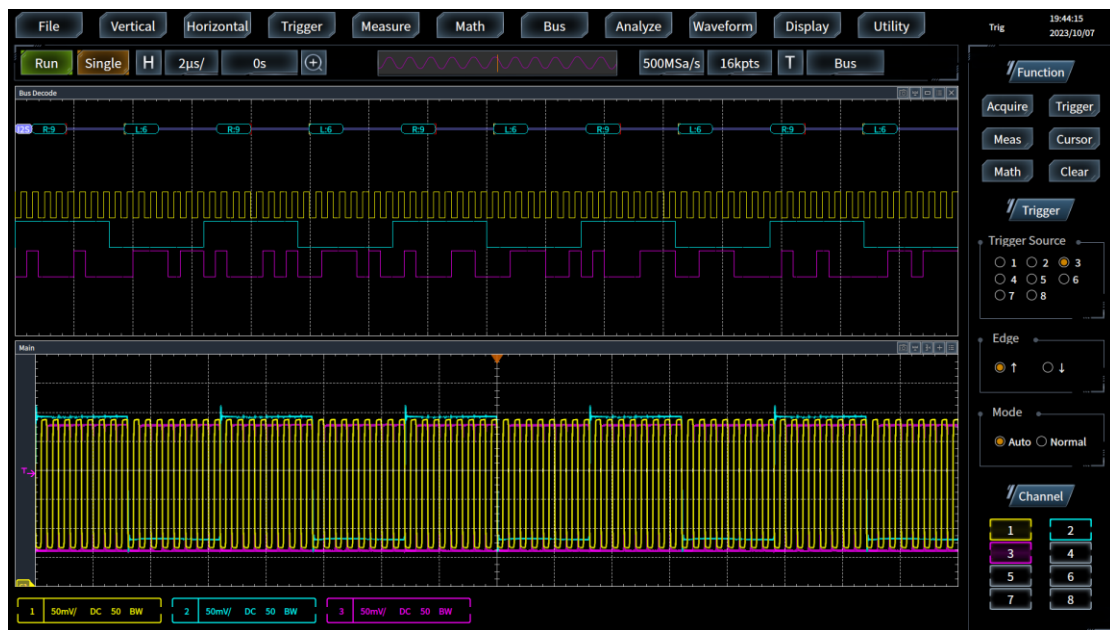
I 2 S, LJ, RJ, TDM audio buses
