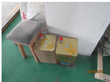
Finding No safety label and secondary container.JPG
