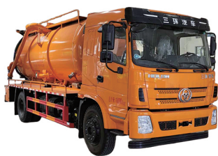
Sewage cleaning truck
