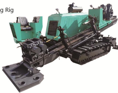
HFDD-100 Horizontal Directional Drilling Rig Max. Pushing Capacity: 102T Max. Rotation Torque: 34000N.m(I Gear)/17000N.m(II Gear) Engine Power: 276kw(2200r/min) Spindle Rotation Speed: 0-110r/min, 0-105r/min
