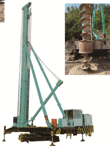
HFXP-50 Crawler Jet Grouting Rig Drill Hole Depth: 50m Drill Pipe Diameter: φ42mm φ50mm φ73mm Borehole Inclination: ± 3° forward tilting 10° backward tilting 90° Maximum Torque: 3000N/m
