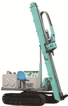
HFJG-6 Crawler Type Hydraulic Anchor Drilling Rig Drilling Diameter: 50-250mm Drilling Depth: 100-120m Input Power: 55kW+ 18.5kW + 2.2kW Rotary Torque : 6800N-m
