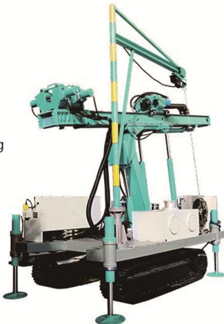
HFJG-6 Crawler Type Hydraulic Anchor Drilling Rig Drilling Diameter: 50-250mm Drilling Depth: 100-120m Input Power: 55kW+ 18.5kW + 2.2kW Rotary Torque : 6800N-m
