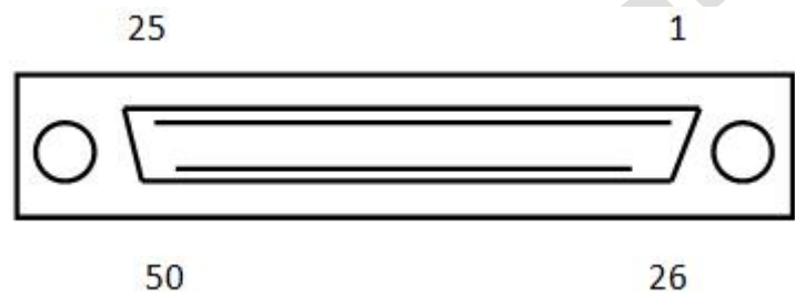
Fig. 8 Description of the ports on the back of the CN1 connector
