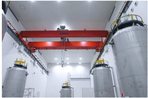
洁净防爆全自动型起重机 Clean Explosion-proof Automatic Crane
