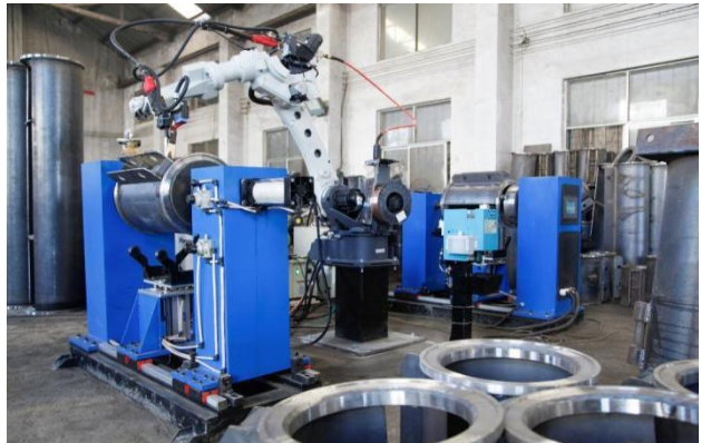
电动葫芦卷筒外罩机器人焊接工作站 Electric Hodrum Cover Robot Welding Workstation
