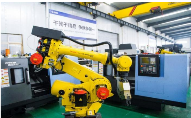
300LD车轮轴智能自动化生产单元 300LD Wheel Axle Intelligent Automation Production Unit
