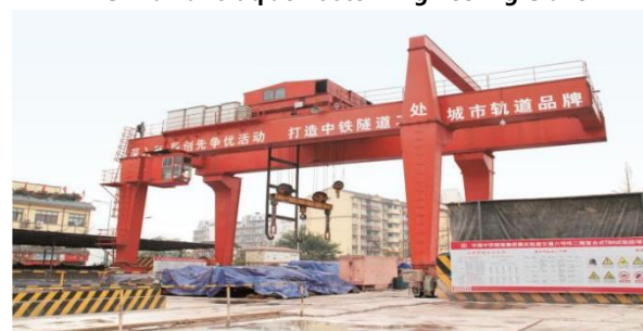
中隧集团重庆轨道交通六号线U型地铁翻渣门吊 China Chongqing Rail Transit Line6 U-shaped Subway Slag Turning Gantry Crane
