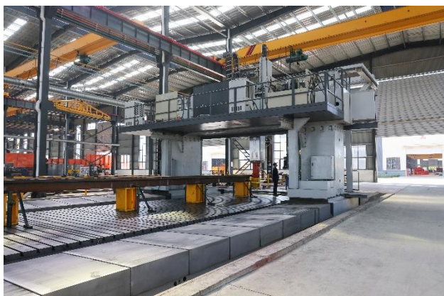
数控定梁龙门移动式镗铣加工中心 CNC Fixed Beam Gantry Mobile Boring and Milling Machining Center
