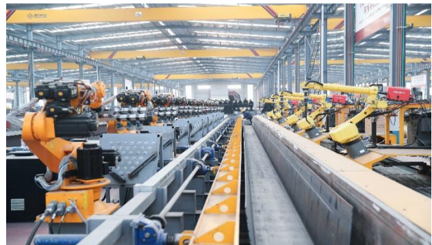
单梁筋板组装焊接工作站 Single-beam Reinforcement Plate Assembly and Welding Workstation
