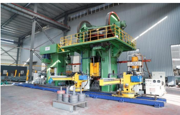
铸钢车间LD轮碾压全自动流水线 Steel Casting Workshop LD Wheel Rolling Automatic Assembly Line
