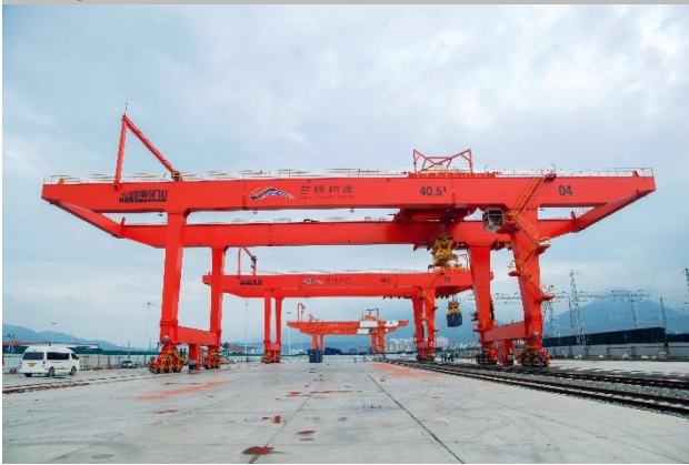
兰铁物流 轨道式集装箱门式起重机 Lantie Logistics Rail-mounted Container Gantry Crane
