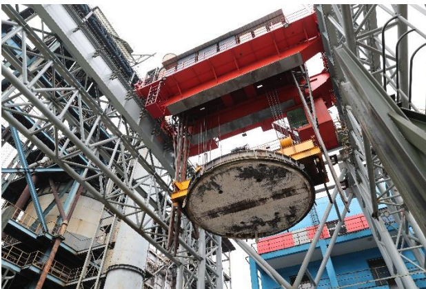
九江迁安 焦罐专用起重机 Jiujiang Qian'an Special Crane for Coke Tank
