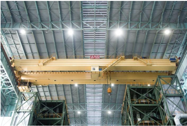
宝武集团全自动无人值守起重机 Baowu Group Fully Automatic Unattended Crane
