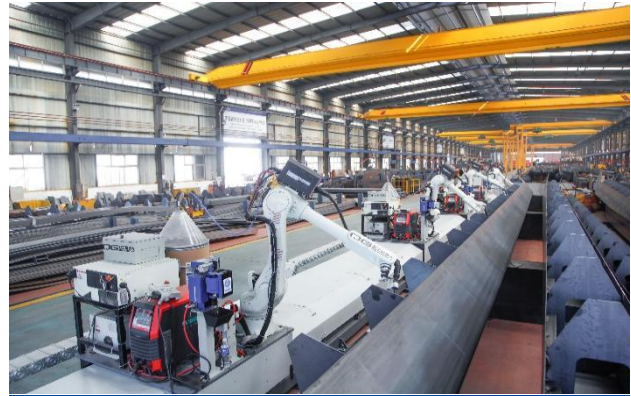
单梁主梁内缝机器人焊接流水线 Robot Welding Line of Single Beam Main Beam
