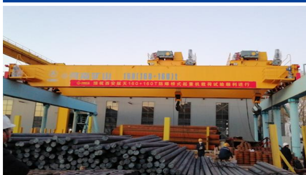
160+160t 防爆双梁桥式起重机 Anti-explosion Double Beam Bridge Crane
