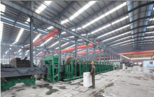
U型槽一次成型生产线 U-groove one-time forming production line
